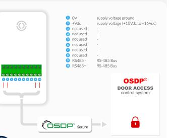
· double-gang back box · As a final check, before fixing the RX5M reader module, confirm you have wired the PIN-OUT connections correctly. Offer up the reader module and securely fix the panel using the M3.5x20mm security screws as supplied. • Run activation / performance test. RX5M reader module
